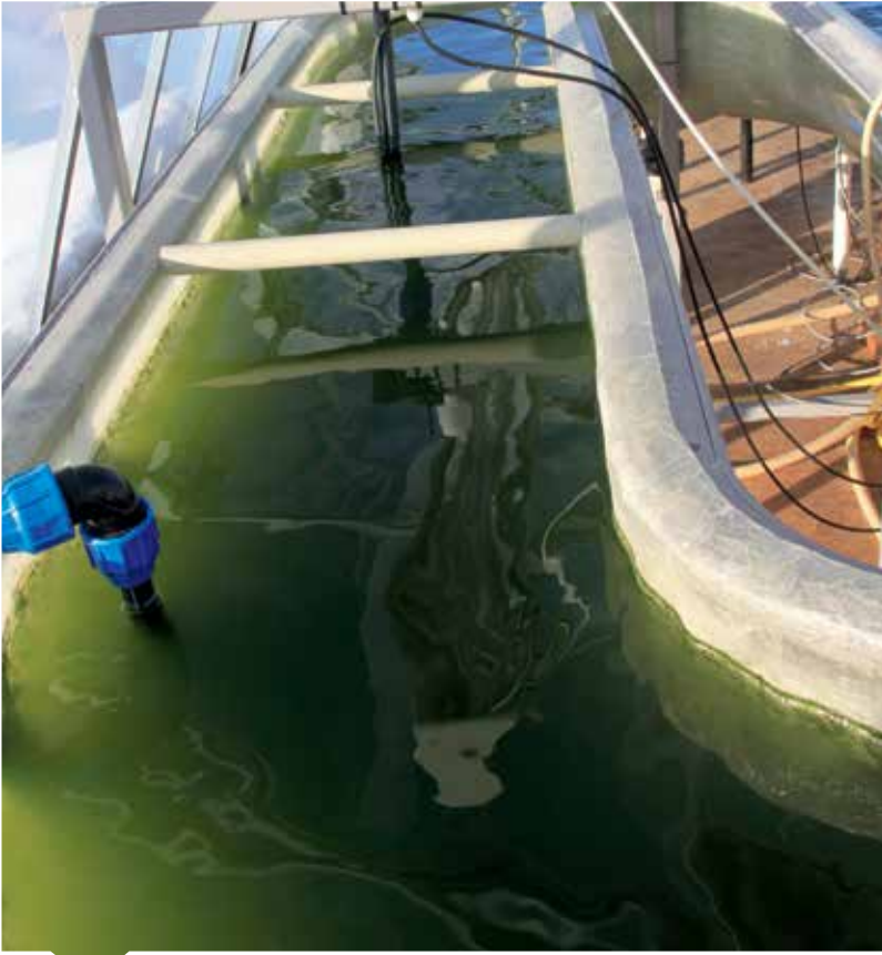
Algae grow well in sewage with the addition of carbon dioxide in flue gases from the power plant. Photo: Francesco Gentili
