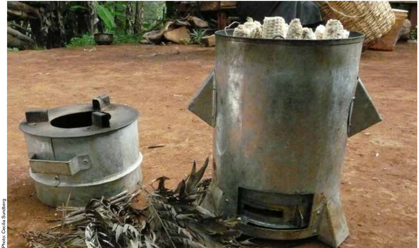
Bio-char producing cookstove with maize cobs as fuel.
