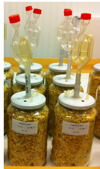
Figure 1 Lab-scale silos with siphons and with stoppers removed for air stress treatment.
