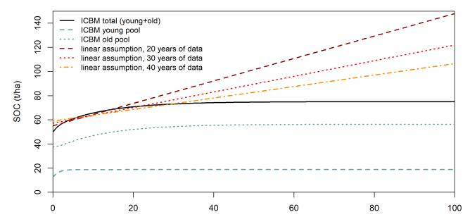
Figure 1: The difference between average sequestration rates (line) and a first-order model (the exponential curve)
