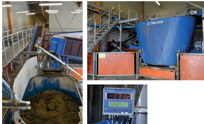
The stationary mixer feeds the conveyor belt feed distributor, but can also be used to load trolleys, feed carts, feed trucks or similar.
