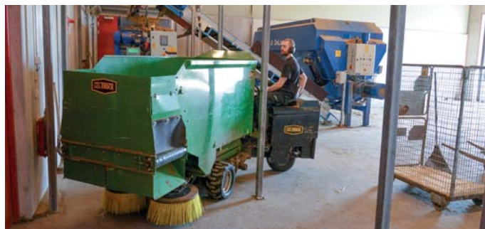
The feed truck can reach practically all parts of the facility and is thus a useful complement. The machine feeds in both directions and is also equipped with a sweeping roller and scissor lift.
