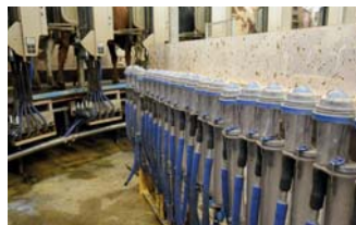
Equipment for milk yield measurement by udder in AMR™.
