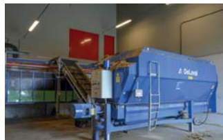
The stationary mixer feeds the conveyor belt feed distributor, but can also be used to load trolleys, feed carts, feed trucks or similar.
