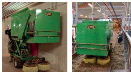
The feed truck can reach practically all parts of the facility and is thus a useful complement. The machine feeds in both directions and is also equipped with a sweeping roller and scissor lift.
