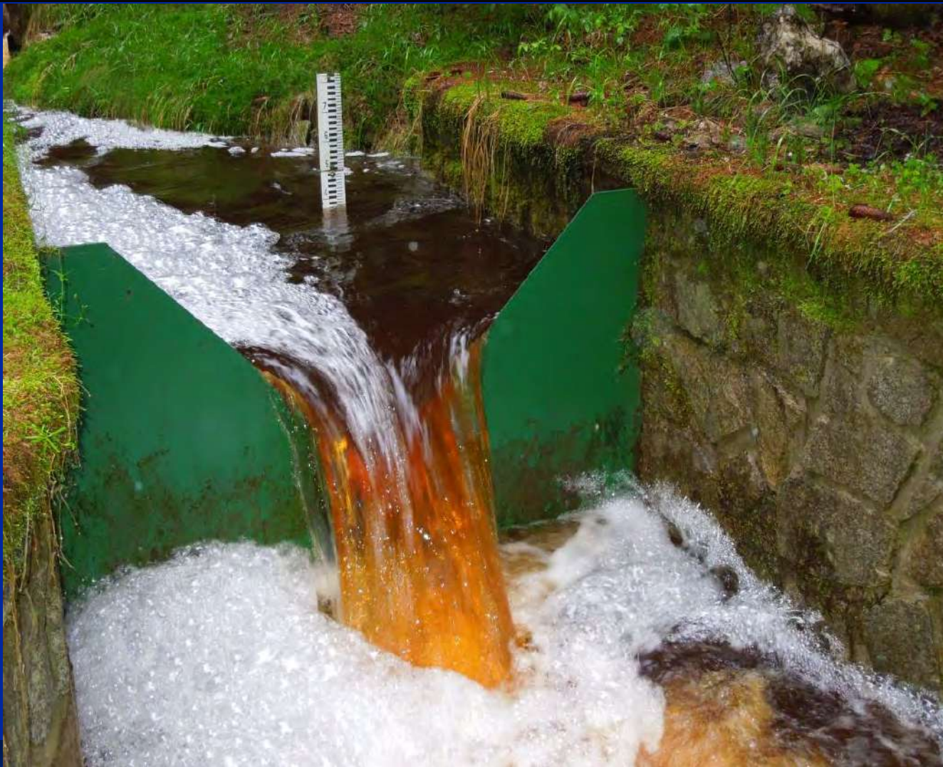
V-notch weir at Lysina during a high flow episode, characterized by brown color due to high concentration of dissolved organic carbon (DOC) generated in shallow water flow paths of forest soils.
