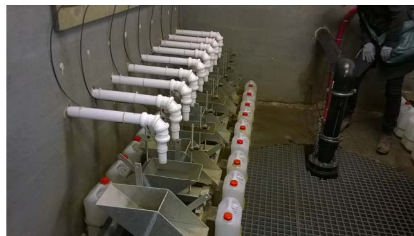
Flow proportional water sampling (Photo: Ole Martin Eklo)
