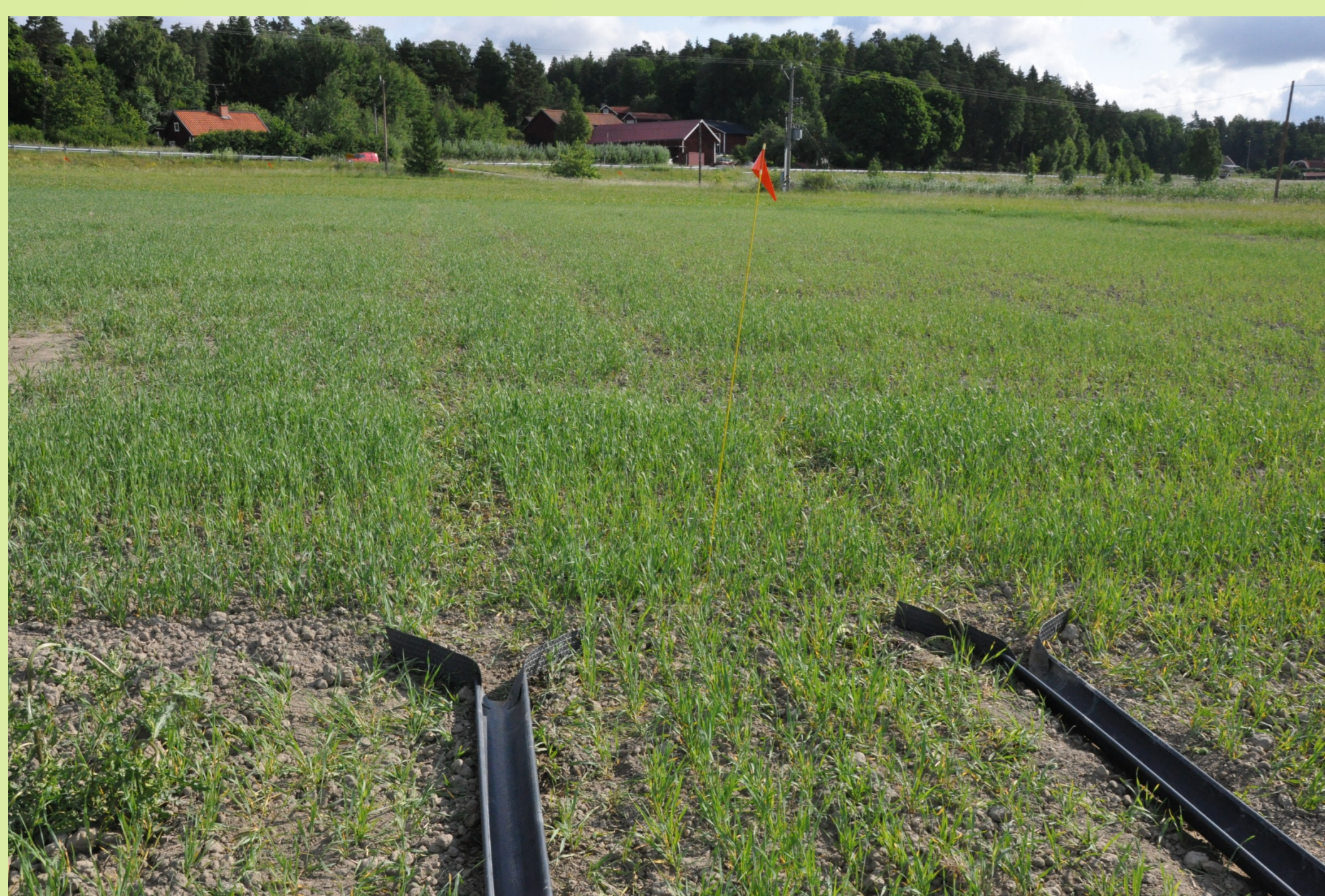
Figure 1. The field site. Surface runoff was collected from wheel tracks during the growing season.
