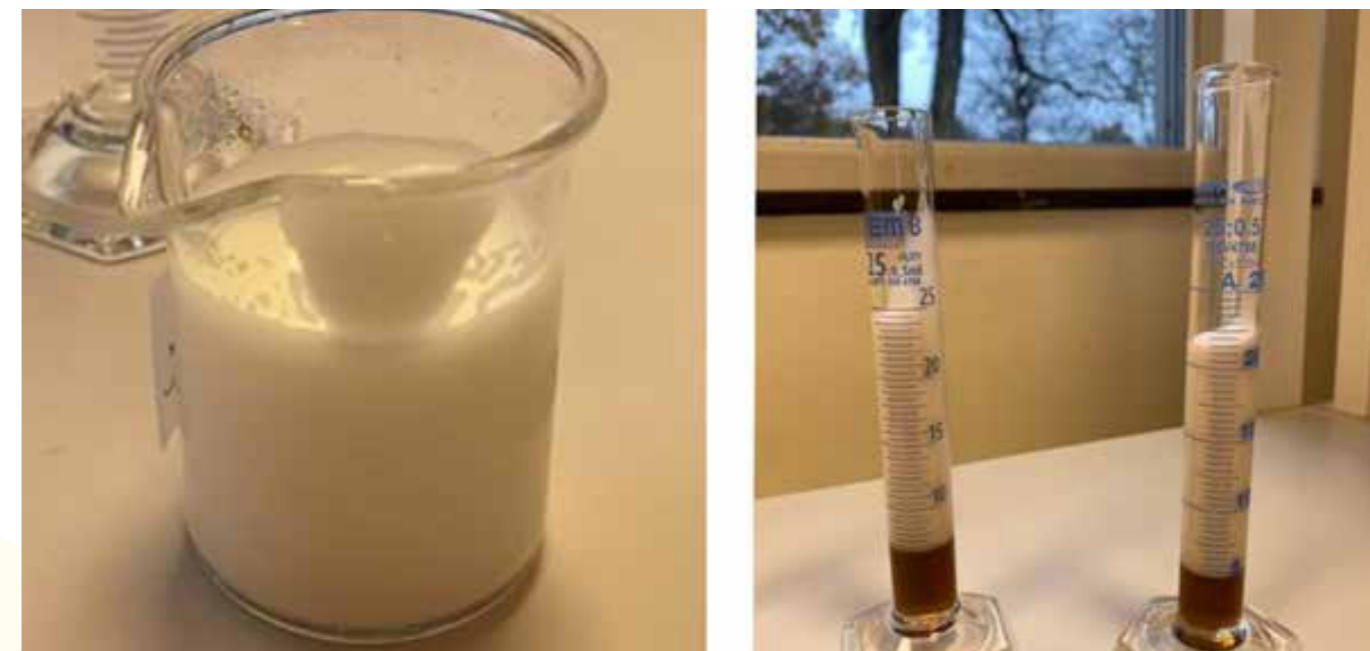
Fig. 4. Foaming capacity of different legume samples after the innovative processing; a) faba bean, b) pea, pre-processed (left) and not processed (right). (Photos by Faraz Muneer).
