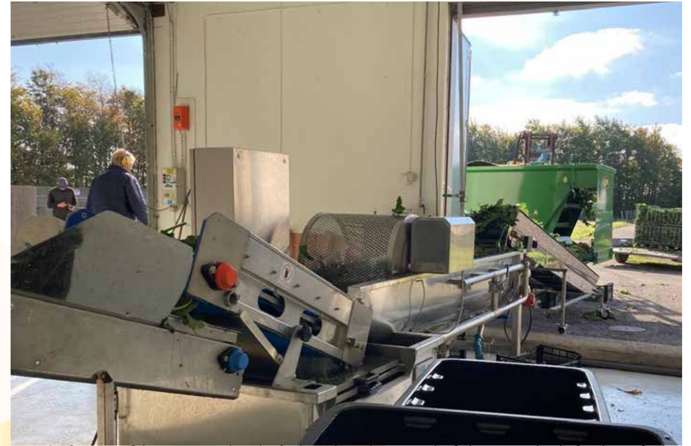
Fig.2 The first part of the process in the pilot facility, where the material is fed into a washer before being further processed. (Photo by Anna-Lovisa Nynäs).
