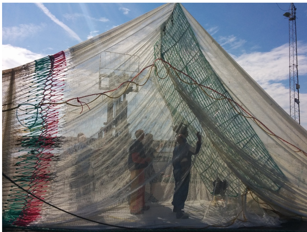
An image showing the assembly of the large grid into the nettings of a pelagic trawl.
