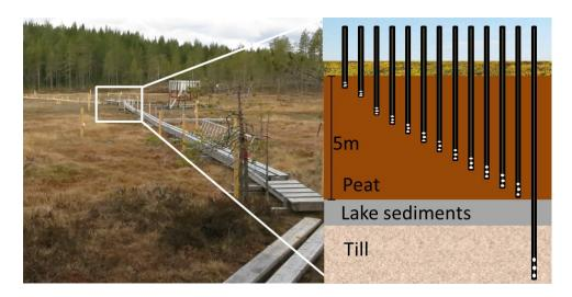
The Kallkäls mire is the source area for stream C4, and the location of the "Russians wells". The "Russian wells" are a set of piezometers allowing sampling at different depth in, and below the mire.
