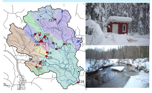
In C7 discharge has been measured since 1980 (above right), C2 and C4 from 1994 and the remaining stations from 2004. The are 18 regularly monitored water quality monitoring *stations* (above left). Six of the stations are in heated houses for year around measurements (left).
