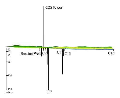
The profile view shows the 150 m ICOS tower and major groundwater wells ranging between 5 and 153m.
