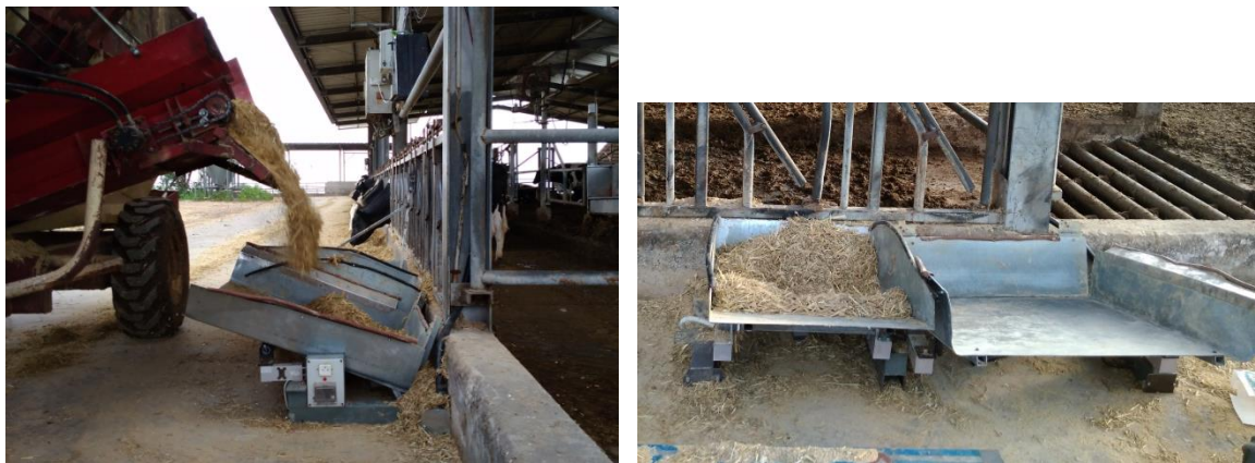
Figure 2 Load cell based systems on the ARO research farm. It is an early prototype that has not been commercialized.
