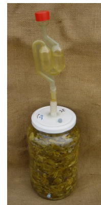
Picture 1. Glass jar silo with water-filled siphon on lid.
