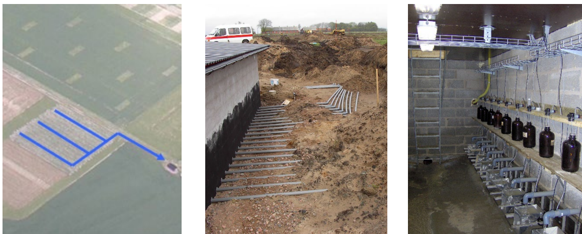
Separate tile-drained plots (left), led to an underground measuring station (middle) with tipping-buckets and flow-proportional water sampling (right). Composite water samples in bottles are emptied every other week and sent for analysis.
