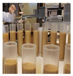
In the Soil Physics laboratory we work with various methodologies for texture analyses, the traditional 'pipettte' method (recommended by the EU Soil Directive to monitor soil health); the PARIO devices, and the so-called Laser Diffraction Methodology (LDM), using particle size determination with reflectance scattering). Initial work comparing these methodologies for Swedish agricultural soils show discrepancies (e.g. Nilsson Nimblad et al 2022; Messing et al 2024).
