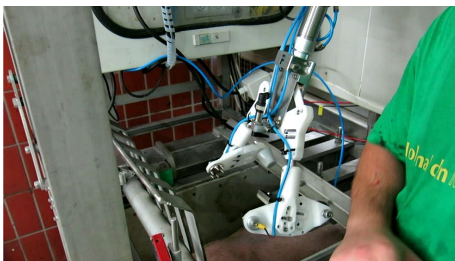
Figure 3.2.3. New semi-automatic pneumatic electrical stunning forceps © M. Marahrens, FLI; © Freund GmbH)
