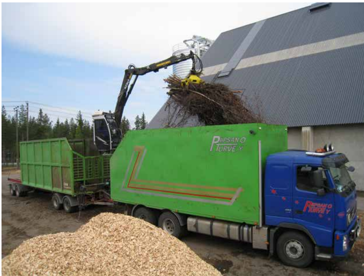
Picture 18. Undelimbed energy wood or loose logging residues can be transported to a terminal or end-users on biomass trucks with covered sides and bottom. (Photo: Juha Laitila)
