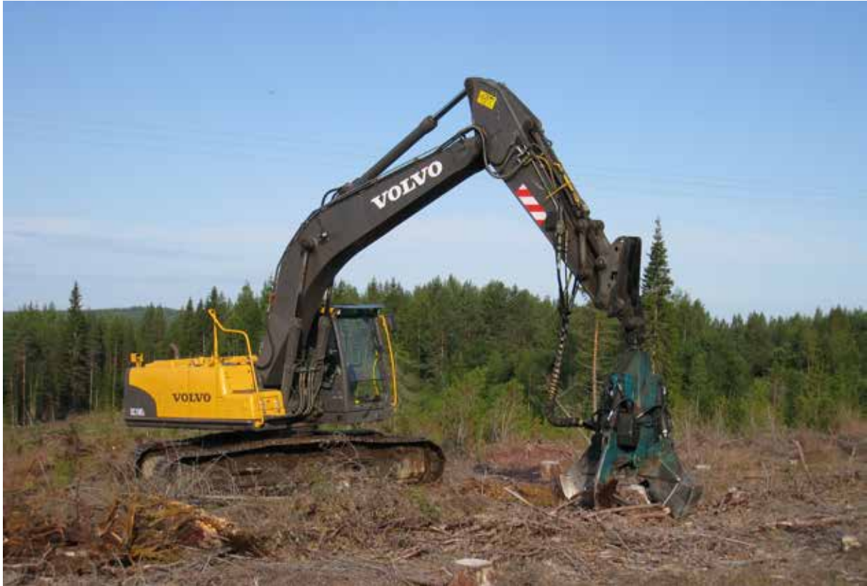
Picture 39. A heavy excavator is stable and strong enough for stump lifting. (Photo: Juha Laitila)
