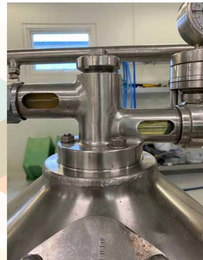
Fig. 1. Bulk centrifugation of precipitate from leaf juice at about 300L/hr. Incoming juice with precipitate on the left and precipitate free "brown juice" on the right. (Photo by William Newson).
