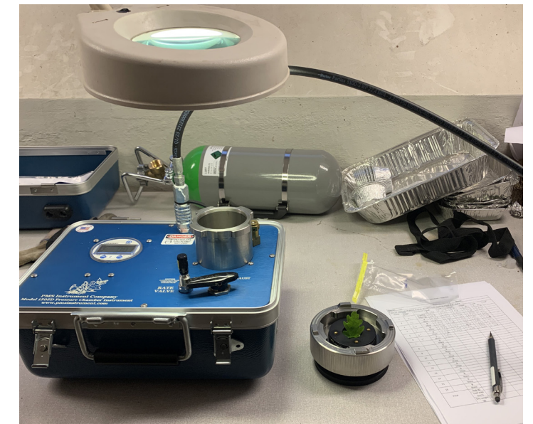
Fig.2: Drought tolerance in leaves can be determined by measuring the turgor loss point. The turgor describes the pressure in the cells, that are somewhat like a balloon, filled with watery cell plasma. By being slightly under pressure, they are pushed against the cellulose cell walls of the plants, keeping the structure stable. When the cells loose water, due to heat or drought, the pressure cannot be kept up and the leaf becomes soft and floppy and wilts eventually. With a turgor pressure meter, the point of turgor loss can be measured.
