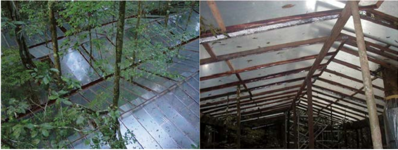
FIGURE 2. The large-scale drought experiment in Caxiuaná, north-eastern Brazil from above (left) and below (right). Rainwater is intercepted by plastic panels (seen from above to the left, and from below to the right) and channeled away from the experimental plot. Photos: Antonio Carlos Lola da Costa.
