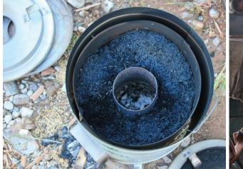
**Figure 1 A.** Small scale biochar production using homemade stove
