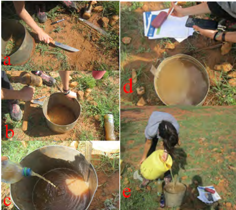
Fig. 18: Procedure infiltration test: a) cleaning the upper part of the soil b) hammering the ring c) saturating the soil d) recording the height according to my chronometer e) refilling with water to reach the initial height (M.Virginia Bile, May 2023).
