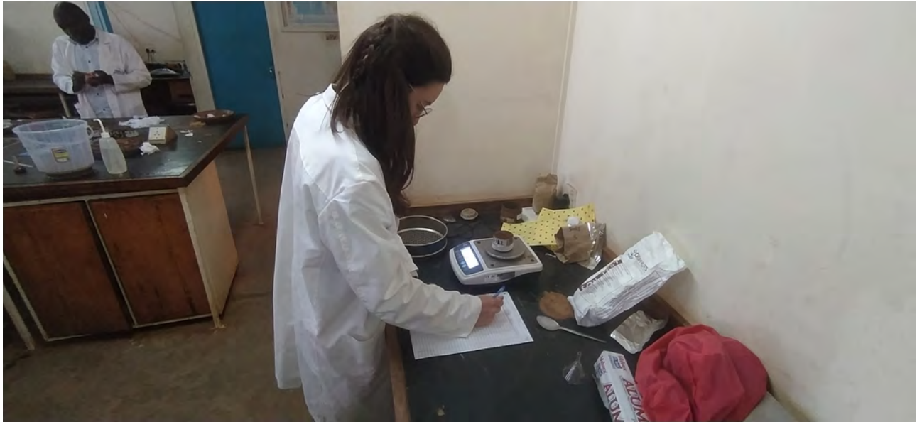
Fig. 13: Measuring the fresh weight of soil samples (M.Virginia Bile, August 2023).
