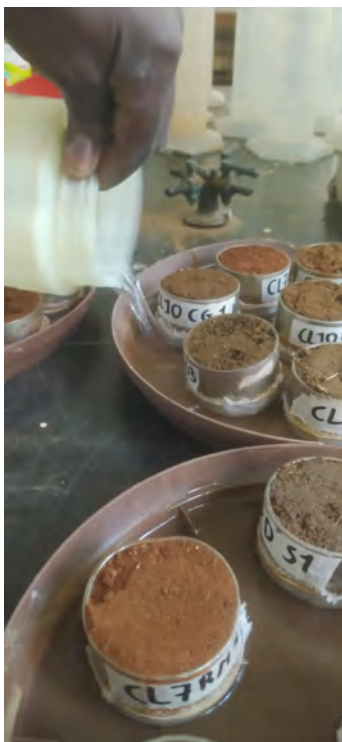
Fig. 14: Saturating the soil sample for 24h (M. Virginia Bile, August 2023).
