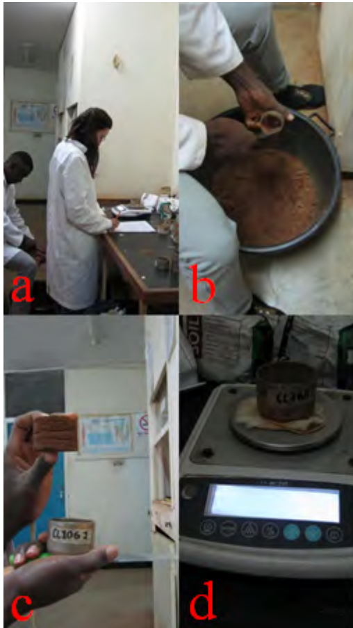
Fig. 16: Weighting the samples after dried and weighting the rings once removed the soil (M. Virginia Bile, August 2023).
