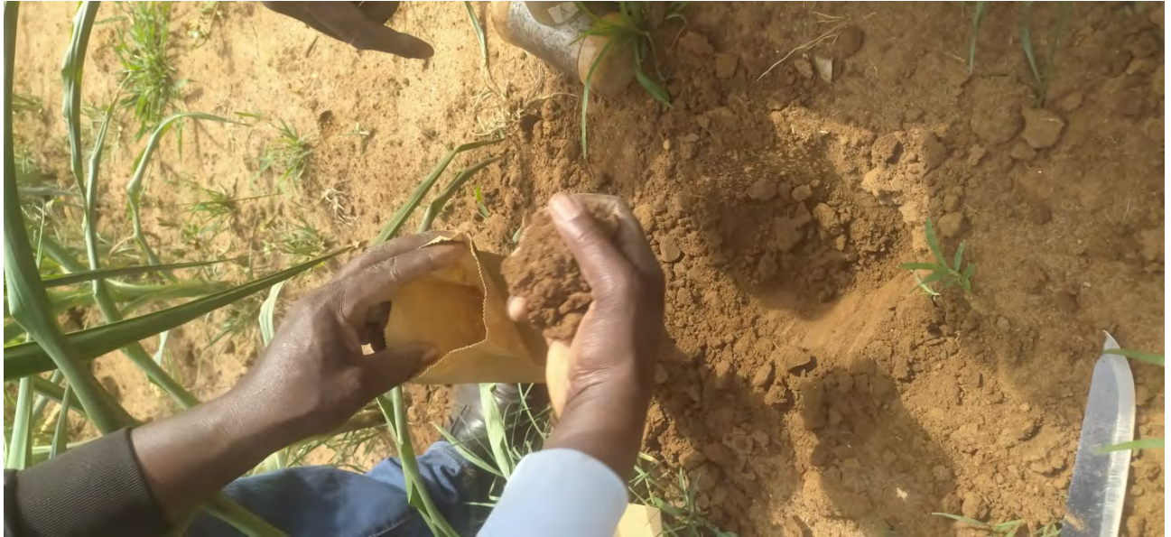
Fig. 17: Collecting soil sample for soil texture analysis (M. Virginia Bile, June 2023).
