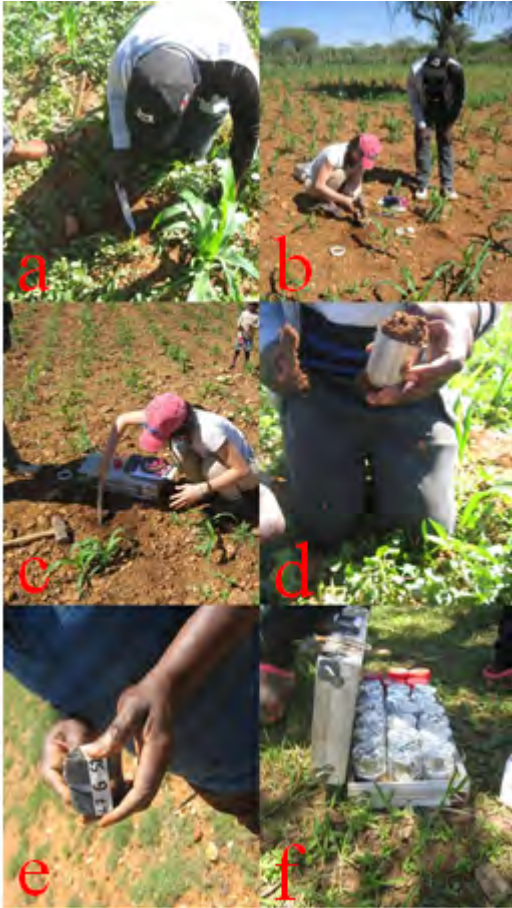
Fig. 12: Procedures soil sampling: a) removing the upper part of the soil b) hammering the ring c) loosening soil around the ring d) extracting the ring with e) closing and labelling the ring f) covered ring with aluminium foil (M. Virginia Bile, May 2023).
