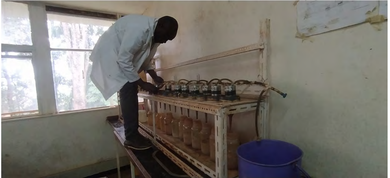
Fig. 15: Ferdinand Anyika-soil physics technician at UoN starting to measure the saturated hydraulic conductivity through a constant head machine (M. Virginia Bile, August 2023).
