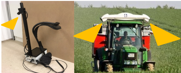
Fig. 2. Left: the hand-held sensor used in this project (Photo: Zhenjiang Zhou). Right: the tractor-mounted Yara N-Sensor (Photo: Yara company homepage). The white instrument on the roof of the tractor is the N sensor, which has an oblique view angle, enabling the estimation of N status on the crop on both sides of the tractor. The yellow triangle in both photos is a depiction of the approximate field of view of the reflectance measurements.
