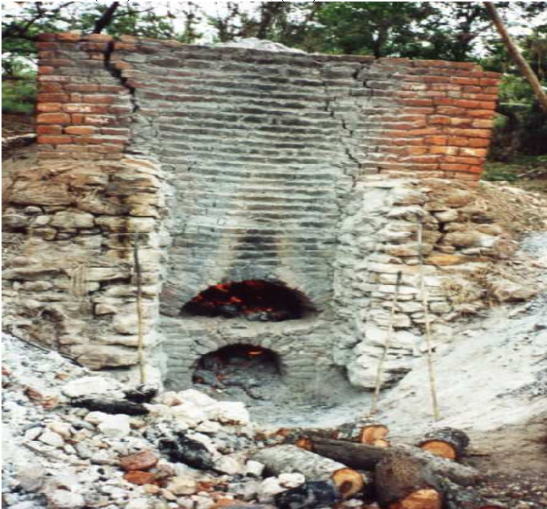
Plate 8: A charcoal kiln inside a village forest reserve in Kasulu, Tanzania. Lime stones are put into the kiln through the top side and are roasted using fuelwood injected below the kiln. Afterwards the stones are cooled and ground to make chalk powder ready for use in house paints or making writing chalks.
