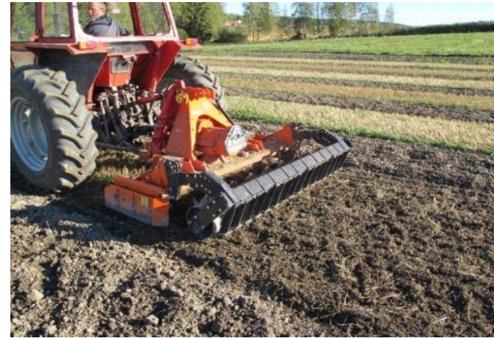
Norway, September 2013: soil tillage using a rotary harrow.
