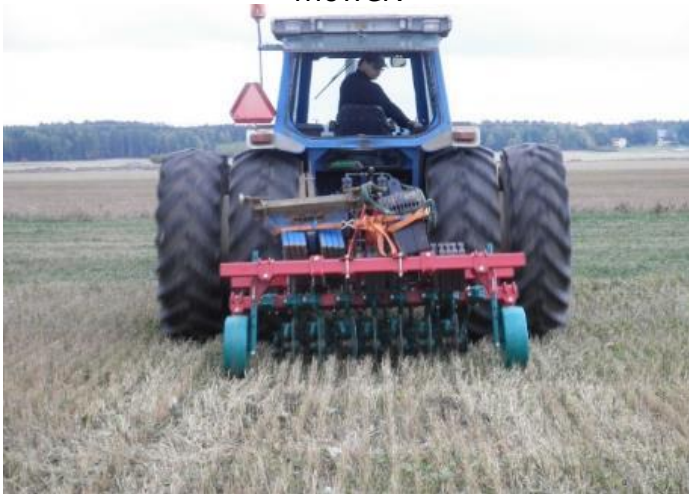
Sweden, September 2013: "Below ground weed control" using the Vertical root/rhizome cutter.
