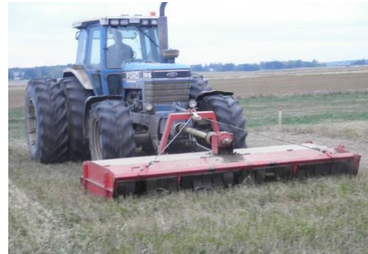
Sweden, September 2013: Above- and below-ground treatments were carried out in the same operation (mowing in front and root cutting behind the tractor).
