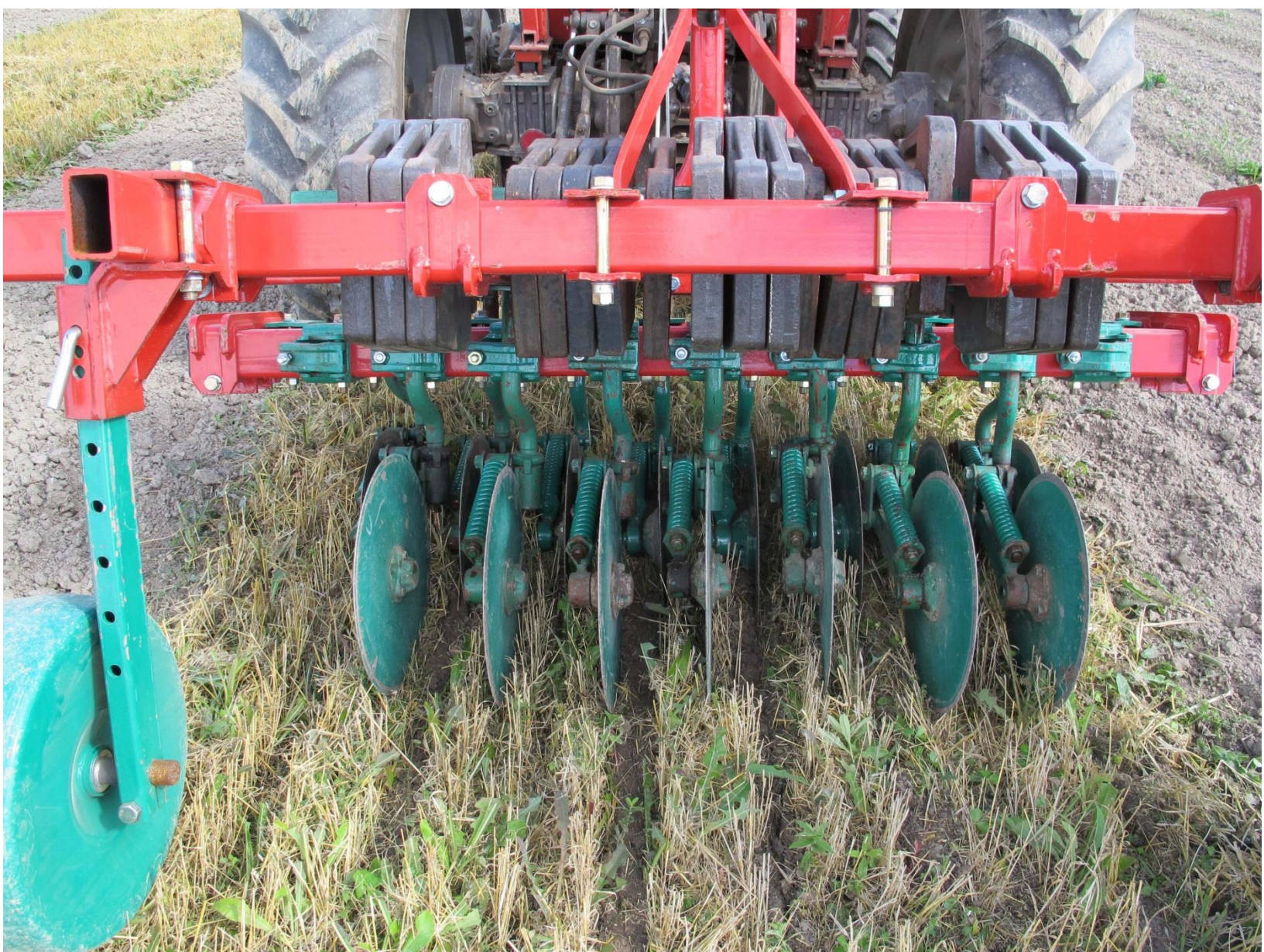
Vertical root/rhizome cutter (“Prototype A” manufactured by Kverneland ASA). 1 Developed for the control of creeping perennials with shallow root systems .
