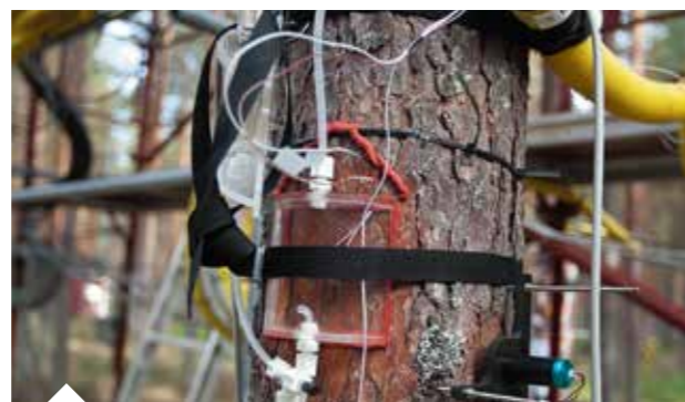
Monitoring diurnal variations in stem diameter.
