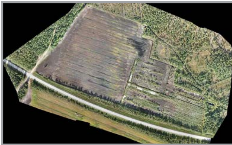
Figure 33. The picture is created from 120 UAV photos by the Pix4D service, and with a flying altitude of 146 meters. (Photo: Alpo Hassinen)
