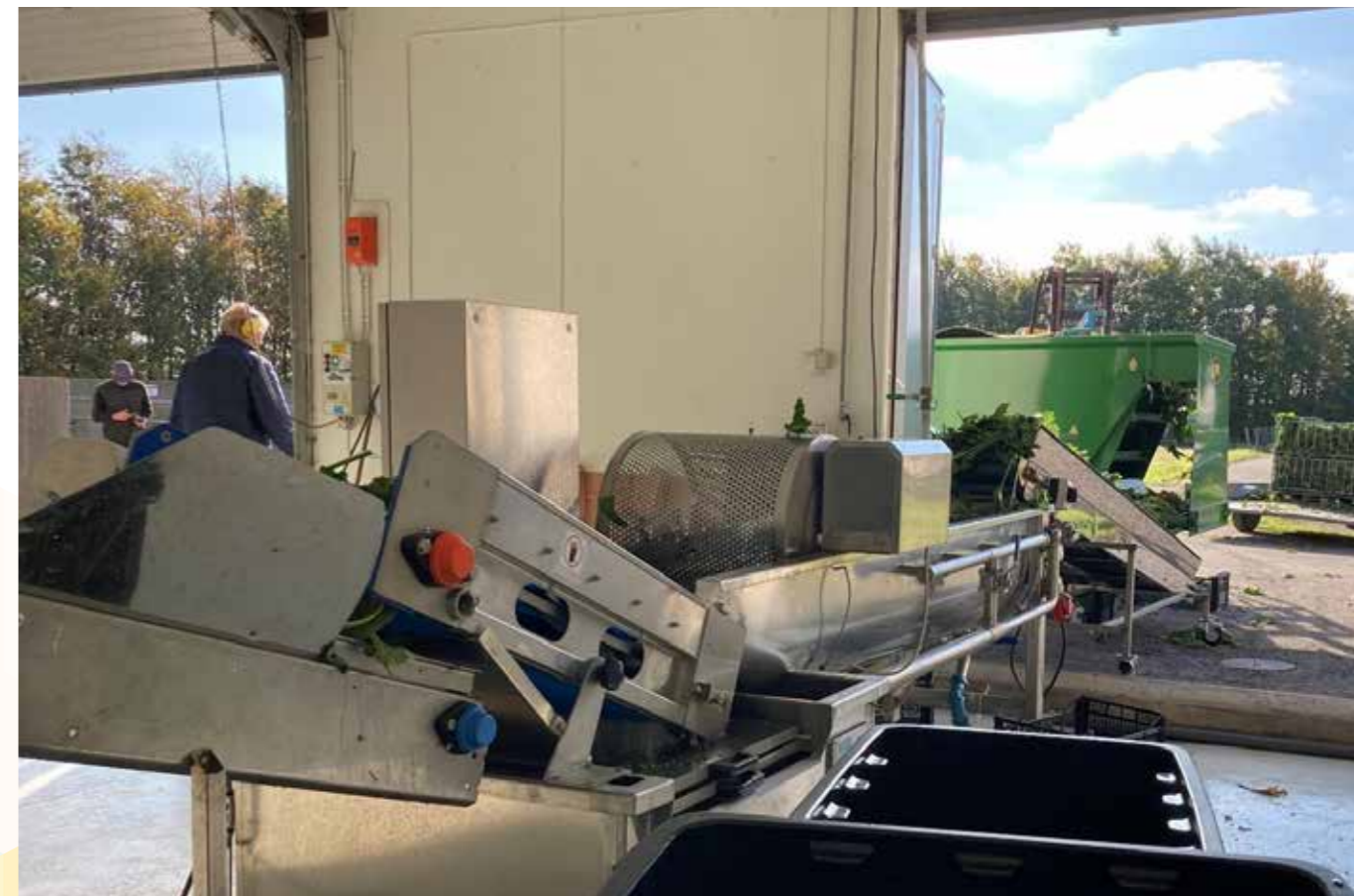
Fig.2 The first part of the process in the pilot facility, where the material is fed into a washer before being further processed. (Photo by Anna-Lovisa Nynäs).
