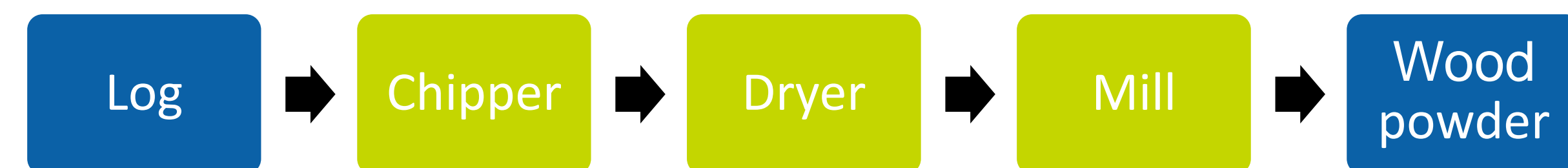
Fig. 1. Conventional pathway to make wood powders relies on intermediate chipping, drying and hammer milling, in addition to handling operations.
