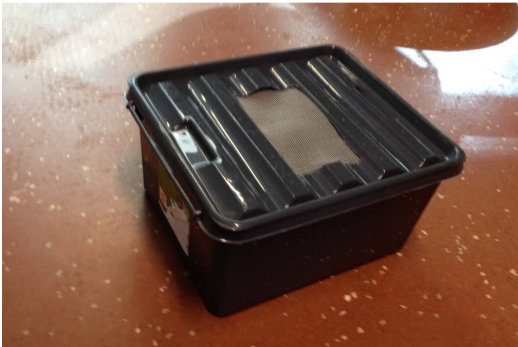
Fig. 2 The SmartStore™ Classic 2 treatment reactor with lid including net for aeration
