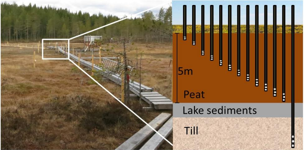
The Kalkäls mire is the source area for stream C4, and the location of the “Russians wells”. The “Russian wells” are a set of piezometers allowing sampling at different depth in, and below the mire.
