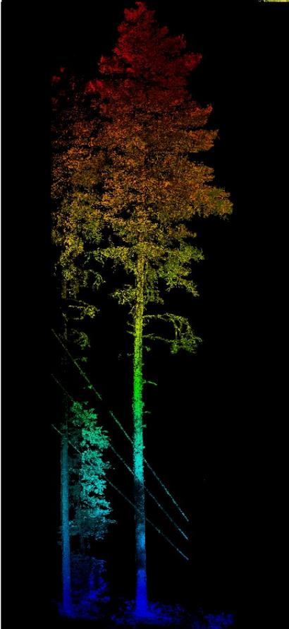
Left: Example of data collected using terrestrial laser scanning using the Trimble TX8 scanner. The picture is a side-view of the three dimensional point measurements of a pine tree at the ICOS tower (note the supporting wires in the picture). Each point is color coded by the height above ground level.
