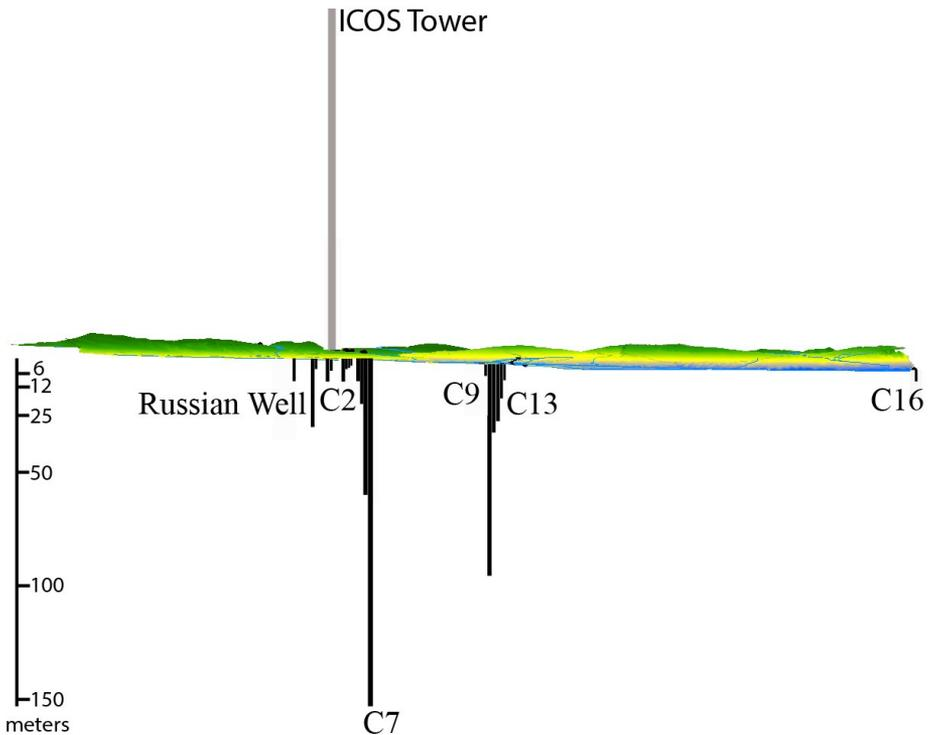
The profile view shows the 150 m ICOS tower and major groundwater wells ranging between 5 and 153m.
