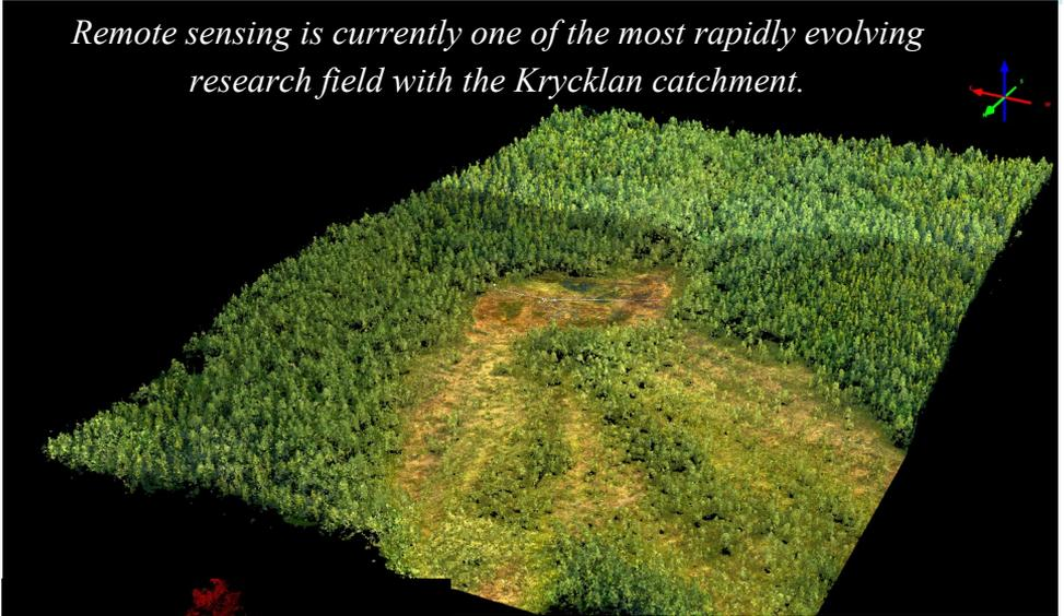
Above: 3D point cloud derived using stereo photogrammetry of very high resolution aerial images. This example is from the Kalkkälsmyren.
