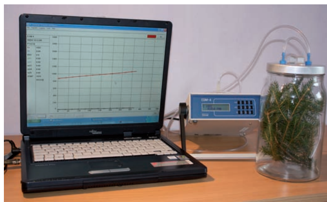
A carbon dioxide analyser from PPsystems is used here with a home-made photosynthesis cuvette. The measurements are simultaneously displayed on a computer.
