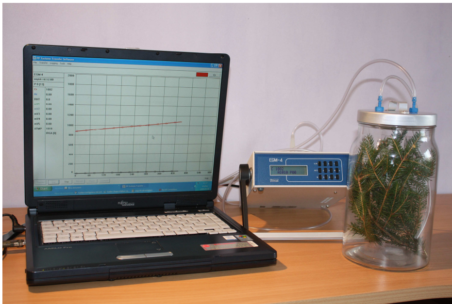
Figure 1. Measurement of photosynthesis and respiration in a spruce twig in low light; the carbon dioxide concentration increases.
