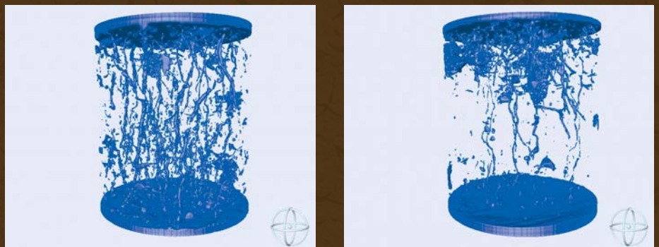
FIGURE 1. Macropores > 0.6 mm in undisturbed soil cores (20 cm height, 20 cm width) collected at 25-45 cm depth in a loamy soil in Skåne, Sweden, with standard management (left) and compacted by a heavy sugar beet harvester 14 years prior to sampling (right). Digitized pictures created from CT-scans by Dr Dorthe Wildenschild (Oregon State University, U.S.).
