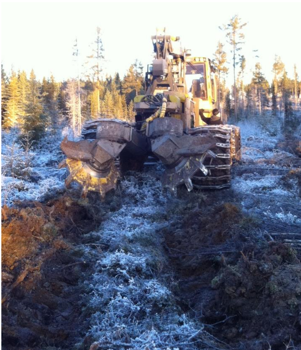
Figure 52: Mechanized site preparation using a Bracke T26 two-row disc trencher in northern Sweden in late November 2018. The trenching unit is mounted on a large forwarder, and the trenching can be performed as long as the soil is not significantly frozen (slight frost and snow is not a problem) (© Back Tomas Ersson, SLU).
