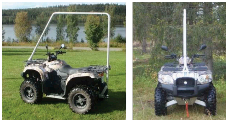
Figure 4. The quad bike and the light ROPS used in Study B.
