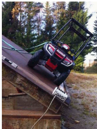
Figure 1. Tilt table with quad bike 1 mounted with the heavy ROPS and positioned at a 0° approach angle (left). Schematic of the tilt table and the four different approach angles tested: 0°, 15°, 30°, and 45°. The tilt table's tilting angle ranged from 0° to 48.5° (Right).
