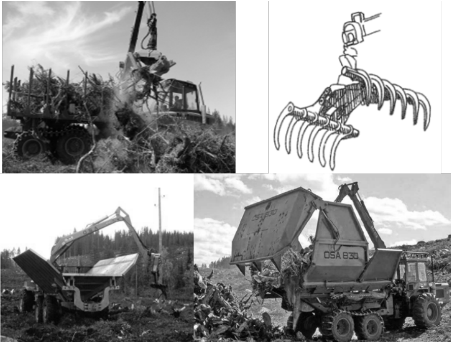
Figure 1. Top left: a current stump forwarder (photo by Kareliatech Oy). Top right: a fork-like stump grapple (From Jonsson, 1985, page 21, figure 20 ). Bottom row: two pictures of specially designed stump forwarders in the 1970-80s (photo by Mats Nylinder).
