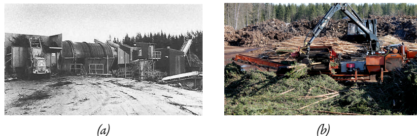
Figure 4: (a) A delibing drum at the forest biomass terminal (Photo: Jonas Palm) (b) Chain flail delimbing at the terminal operations.
