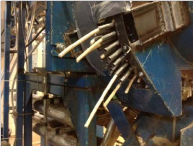
Figure 15. Prototype sampling device ( 8 \times 3 ) for the SPC PP300 Compact Pelletizer (Photo: M Rudolfsson).
