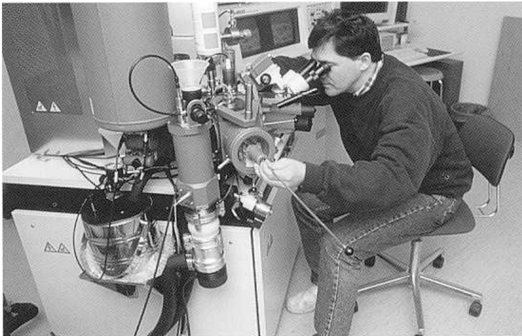
The new high resolution Field Emission Electron Microscope (FE-SEM).
