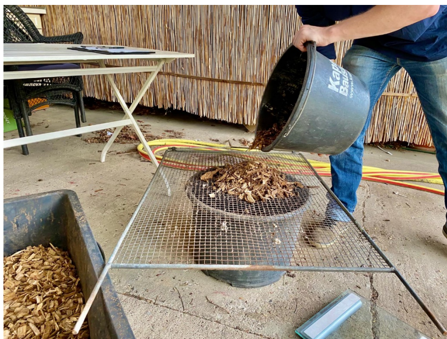
Figure 18: Sieving of wood chips for simplified analysis of particle size – quality assessment on the premises of Castle Property Altlandsberg; picture: S. Ruebsam
