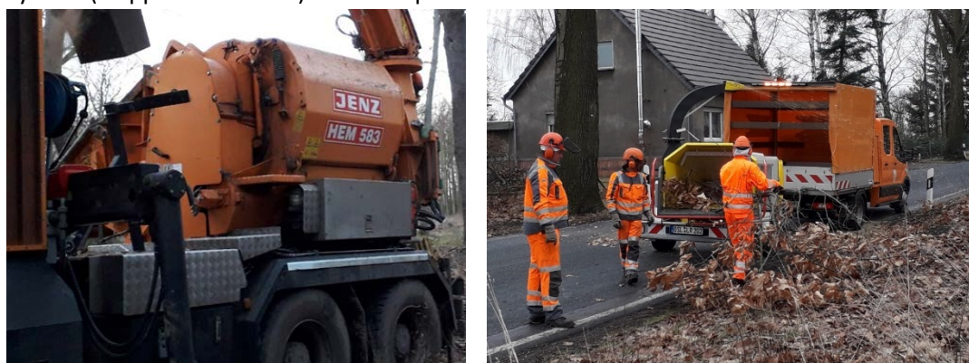
Figure 12: Drum chipper in detail (left) and common technology and work flow for processing material from trimming trees at the road side (right); pictures: M. Schultze
