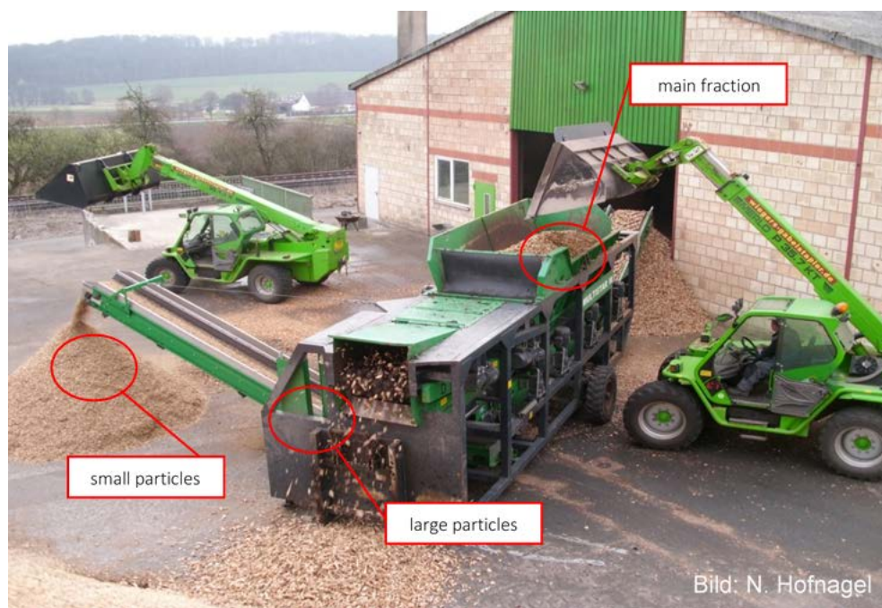
Figure 17: Mobile star screen for separating three fractions, picture: N. Hofnagel
