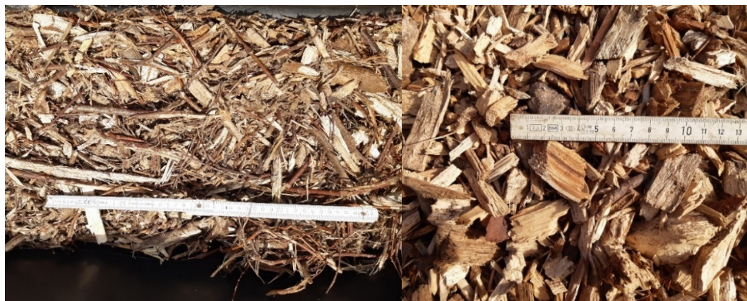
Figure 11: Wood chip quality according to used rawmaterial: left: wood chips from harvesting small trees under power line near Altlandsberg; right: wood chips from felling trees for lanscape preservation; pictures: H. Hartmann
