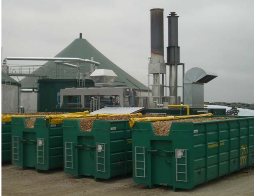
Figure 15: Batch drying in modified bulk containers using heat from a biogas plants; picture: www.energieholz-brune.de
