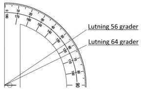
When SRT306/SRT326 is in a position tilted at least 64 degrees, a timer will be activated. When SRT306/SRT326 has been tilted at least 64 degrees for 25 seconds, the SRT306/SRT326 will warn that an alarm soon will be sent off to Securitas. The warning is a sharp signal lasting for 25 seconds. If the SRT306/SRT326 is not straightened back up to at least 56 degrees during these in total 50 seconds, the unit will send off an alarm and call Securitas.
