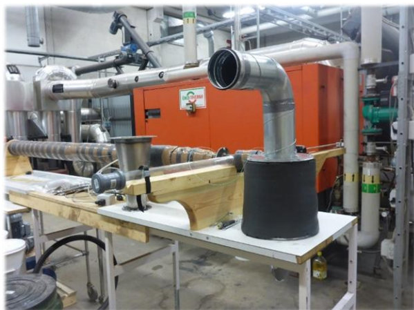
Cyclone dryer For wet and sticky materials
