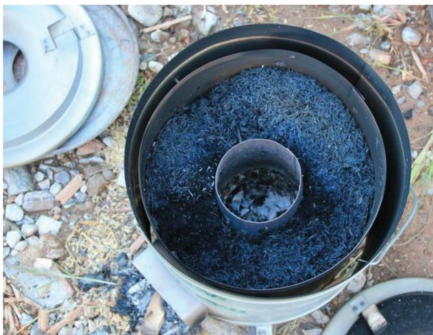
**Figure 1 A.** Small scale biochar production using homemade stove
